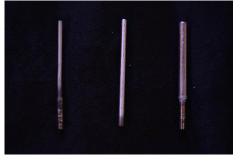
Figure 12. Picture of the three different diameter of inner conductor: 1.2, 1.7, 2.3 mm.
