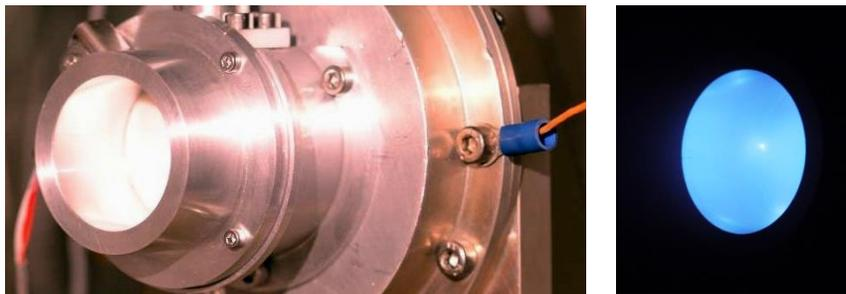
**Figure 6. Picture of the waveguide thruster (left) and its plasma (right).**
